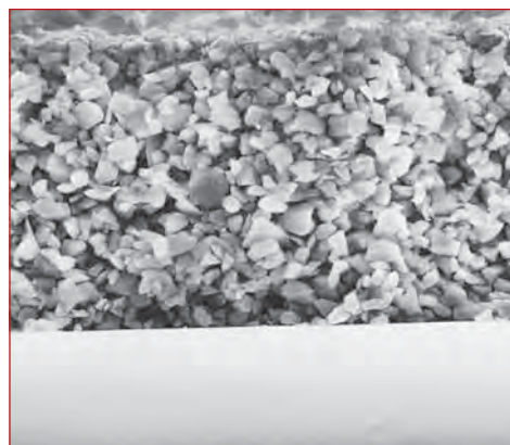
Electron microscopic photograph of a cross section through a glass plate with silica layer (magnification x 500)
