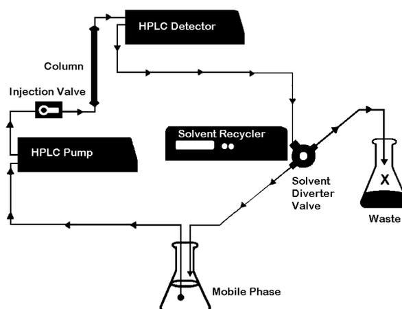
*The Solvent Recycler is compatible with any isocratic liquid chromatography system.*
