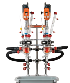
Similar vessel sizes with single circulator manifold kit
